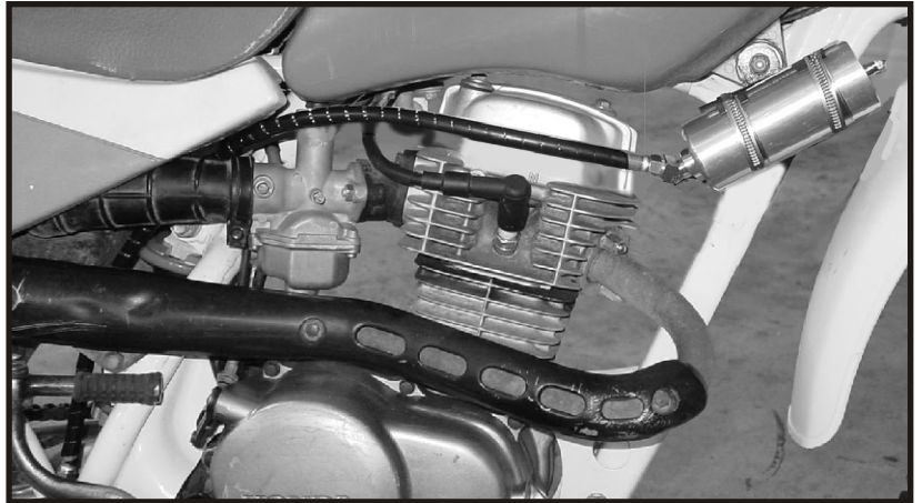
Fig.1 Hose goes up to the left of the carburetor intake boot and to the right of the carb top. The hose should make a smooth arc. Early model shown. Bracket is attached to tank mount. Do not zip tie, wire or clamp the hose to any part of the motorcycle, as the hose should be allowed to move up and down as the suspension moves.
