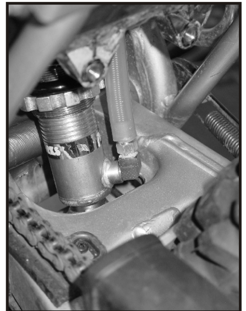
Fig.2 Hose exits to the right rear. After Aug. 1, 2003 all XR shocks were produced with a threaded body with a flush mount. Earlier welded shock is shown.
