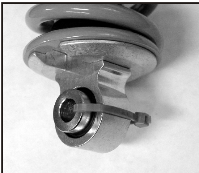
Fig. 2-- Spherical bearings eyelets are fitted with steel sleeves that are 3/4-inch in diameter and look like this. It may be helpful during installation to leave the zip ties on until the eyes are partially centered in the channel.
