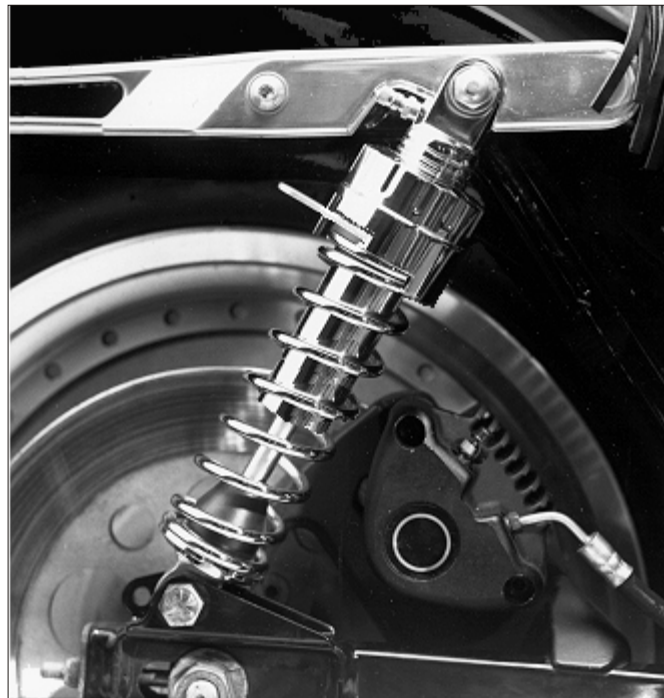
Fig. 2-- Shock compressed with the ARS lever in the softest position. The deepest slot allows the spring set to stay softer longer. The shallowest slot allows the spring set to get stiffer sooner.
