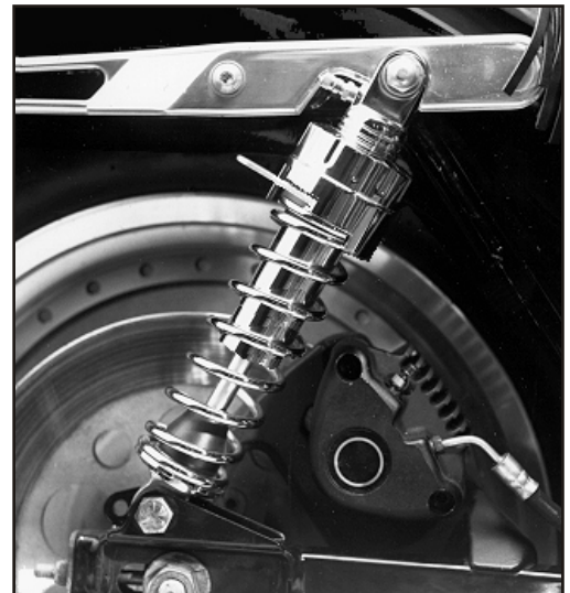
Fig. 1-- Typical installation. Note that the shock body is at the top with the shaft pointing down. Shock shown has optional billet ARS option.
