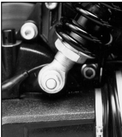
FIG. 3. PRELOAD ADJUSTMENT NUT (PARALEVER ONLY)
