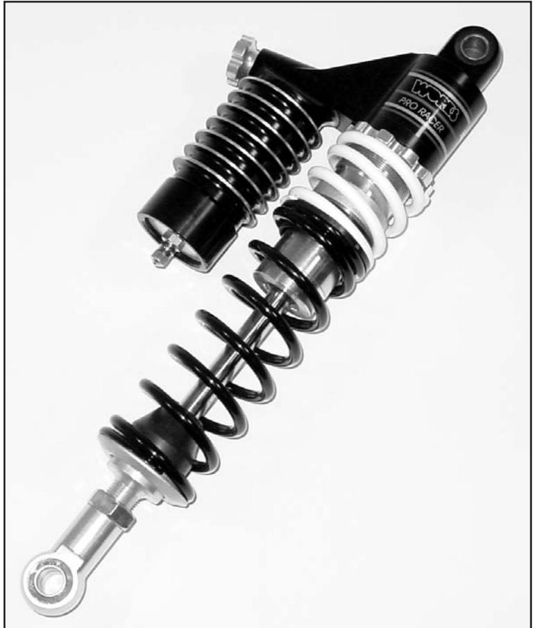
Fig. 1: Pro Racer rebound and compression damping adjustable shock also features threaded spring pre-load and-- in some applications-- ride height adjustment with adjustable length eye (shown).
