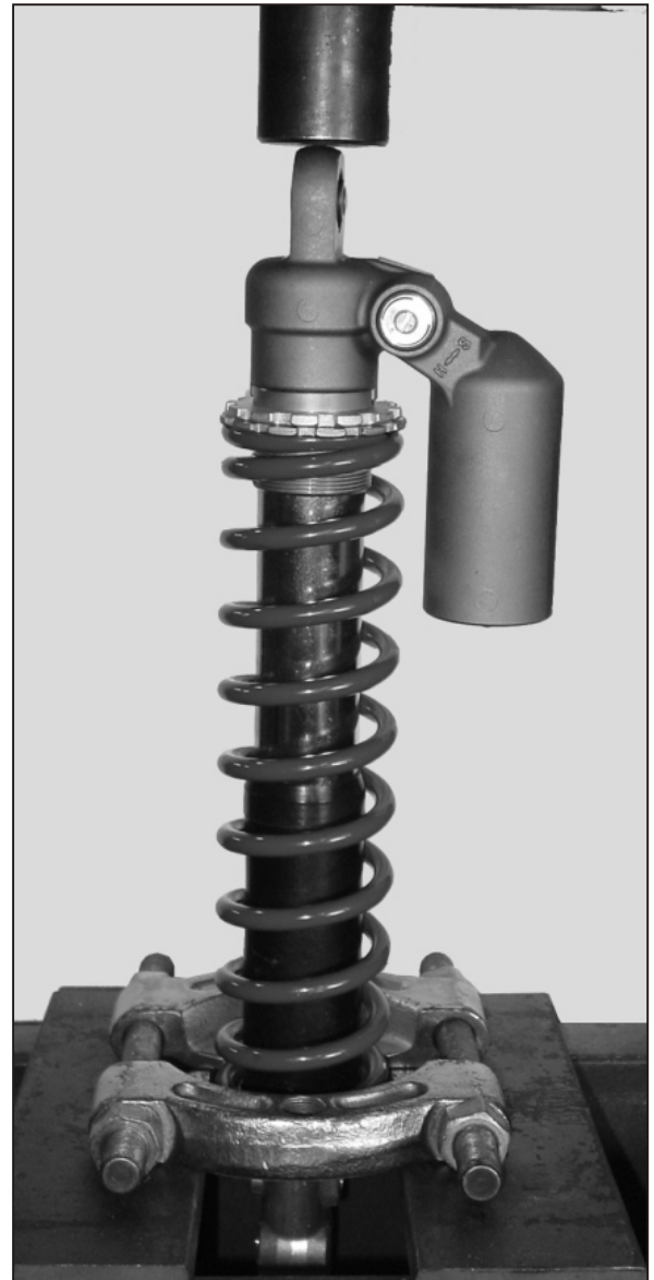
Fig. 3-- Run the ram down on the end of the body eye to push the shaft end eye through the split retainers, allowing the retainers to be removed.
