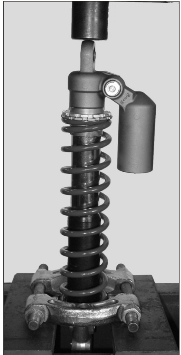
Fig. 3-- It may be necessary to remove the springs using a hydraulic press and bearing press, depending on the application. Run the ram down on the end of the body eye to push the shaft end eye through the split retainers, allowing the retainers to be removed. Typical shocks and press set-up shown.
