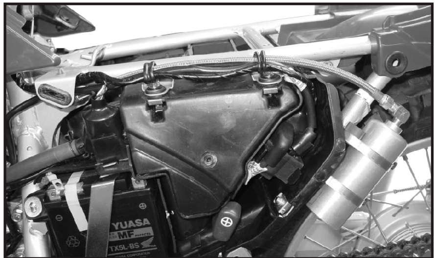
Fig. 2. View of the hose routing over the airbox. The hose then arcs over the top of the air box along side the wiring loom. The non-adjustable reservoir (shown) has a 90 in the top. The hose for the adjustable compression reservoir goes into the back, but the mounting location is the same.
