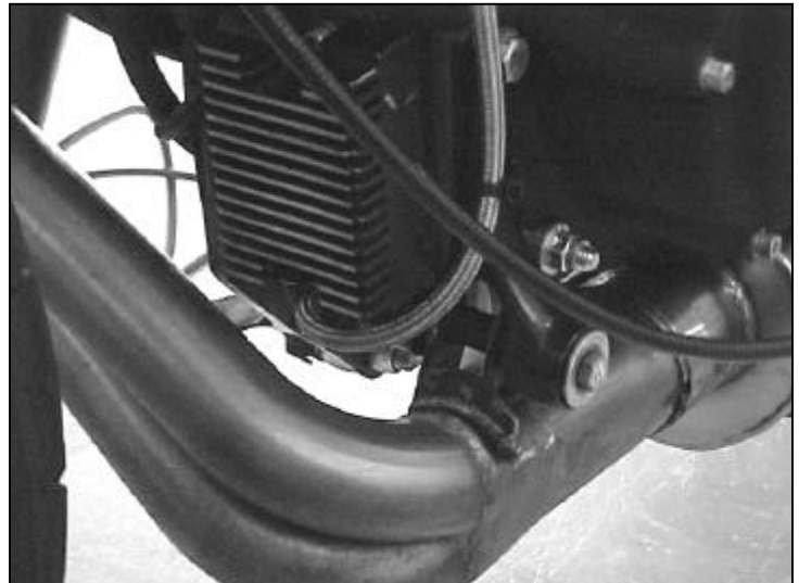
Fig. 3: The hose should exit at the front of the bike and to the left of the engine mount. Use zip ties to keep the hose away from the pipes.
